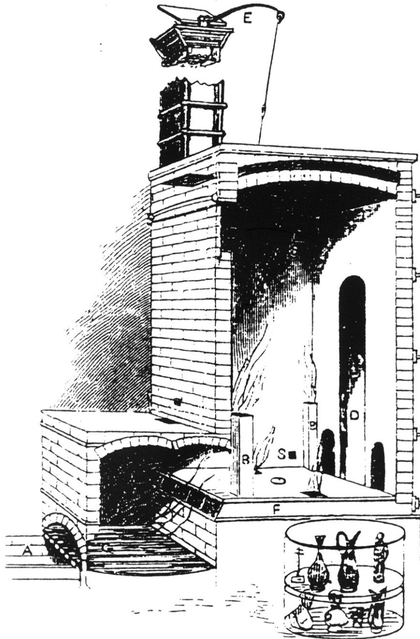
Fig. 29. — Broome's Improved Porcelain or Parian Kiln. A, ash-pit; G, grate; F F, flues; B B, bags for the flames; D, door for filling the kiln; E, damper, or draught regulator; S S S, spy-holes for watching, or trials while burning.
